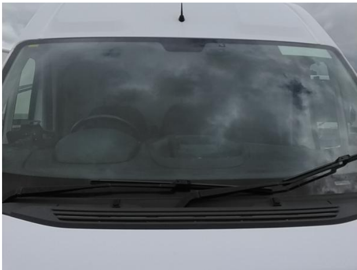
3: Screen Front Chipped Over 10mm
