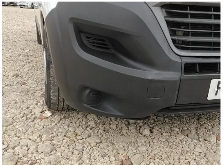
4: Bumper Front Dented 2 Or Less UpTo 10mm
