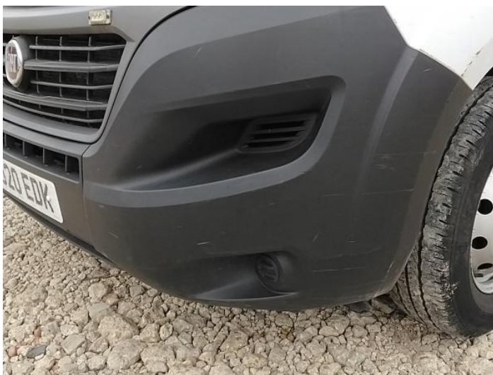
5: Bumper Front Moulding Scuffed (Unpainted) Over 100mm
