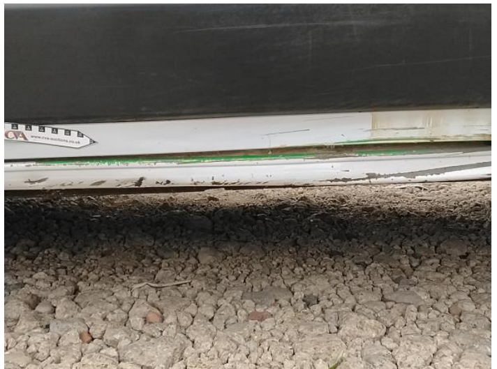
12: Door nsr Dented With Paint Damage
