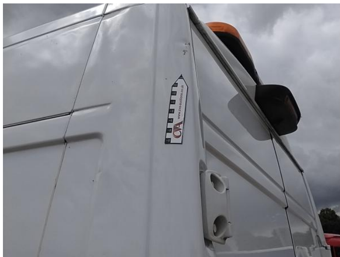
16: Qtr Panel nsr Dented With Paint Damage
