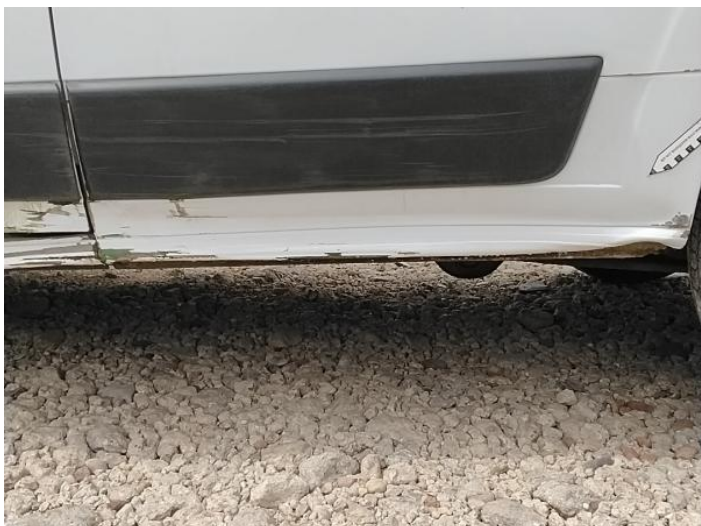
15: Sill ns Dented With Paint Damage
