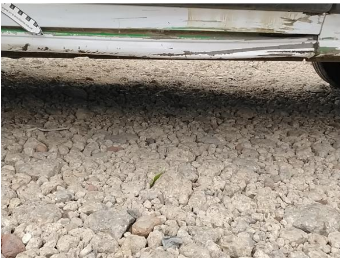
13: Sill ns Dented With Paint Damage
