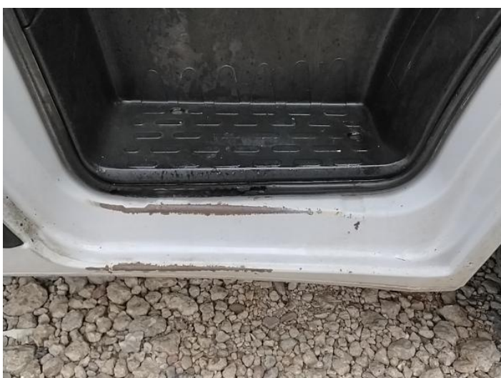
19: Sill os Rusted Over 5mm
