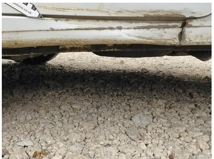
8: Sill ns Dented With Paint Damage
