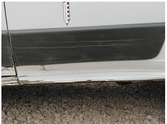
14: Qtr Panel Moulding ns Scuffed (Unpainted) Over 100mm
