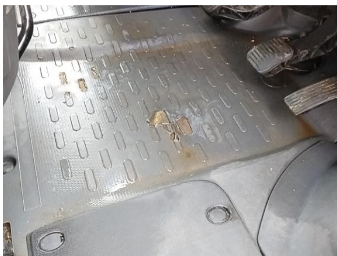
20: Seat Base Cover osf Holed Over 3mm
