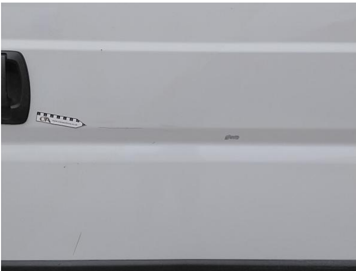
11: Door nsr Scratched Over 25mm Thru Paint
