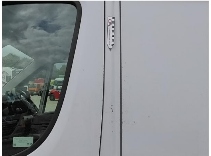
10: B Post ns Chipped Multiple Chips
