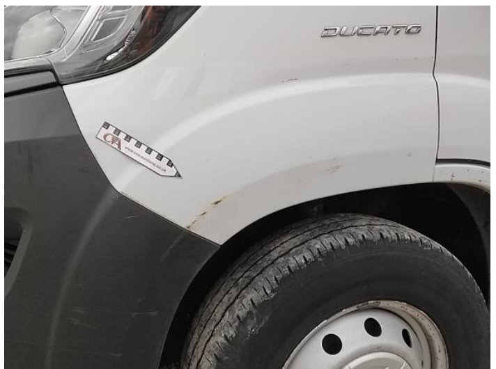
6: Wing nsf Scratched Over 25mm Thru Paint
