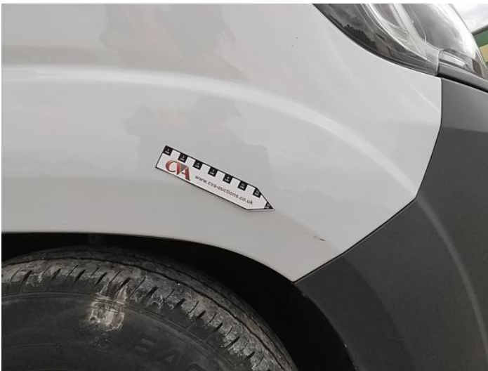
1: Wing of Scratched Up To 25mm Thru Paint
